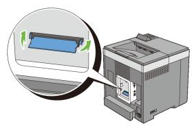
5 Hold the memory module and pull it straight out.
